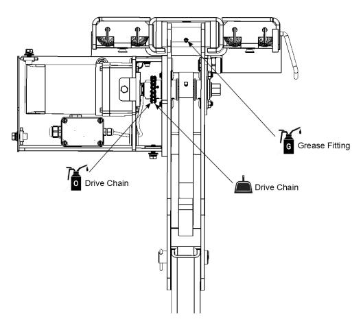
Figure 5: Lubrication and cleaning points (Top View)
