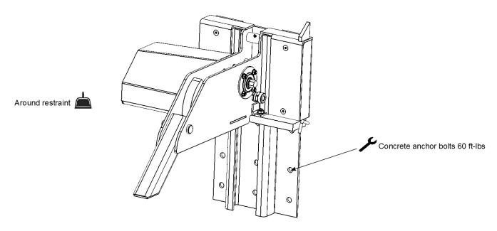
Figure 7: Anchoring and cleaning points
