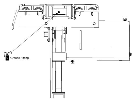
Figure 6: Lubrication point (Bottom View)
